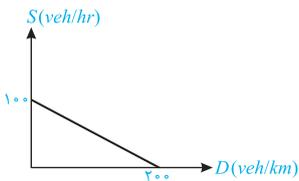
$$S = a - (bD) \Rightarrow \begin{cases} \text{اگر } D=0, S=100 \text{ km/hr} \Rightarrow 100 = a - (b \times 0) \Rightarrow a = 100 \\ \text{اگر } S=0, D=200 \text{ veh/hr} \Rightarrow 0 = 100 - (b \times 200) \Rightarrow b = 0.5 \end{cases}$$
