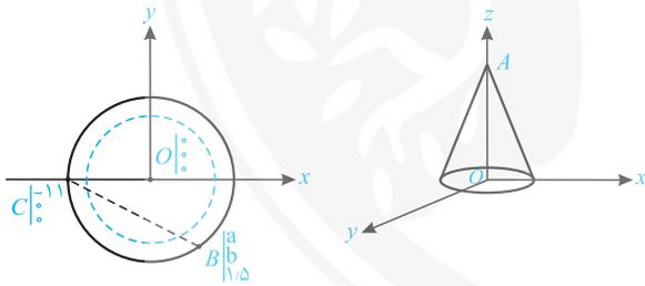
$$\left\{ \begin{array}{l} \text{معادله خط BC در فضا: } \frac{x-x_1}{a} = \frac{y-y_1}{b} = \frac{z-z_1}{c} \Rightarrow \frac{x+11}{a+11} = \frac{y}{b} = \frac{z}{1/5} = r \quad (I) \\ \text{معادله کلی مخروط: } \frac{(x-x_0)^2}{m^2} + \frac{(y-y_0)^2}{n^2} = \frac{(z-z_0)^2}{t^2} \quad \xrightarrow[x_0=y_0=0]{m=n=1} x^2 + y^2 = \frac{(z-z_0)^2}{t^2} \quad (II) \end{array} \right.$$
