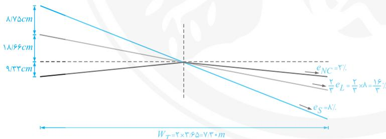
$$\Delta h_1 = \frac{W_T \times e_{NC}}{200} = \frac{7 \times 215}{200} = 1175 \text{ cm} \quad , \quad \Delta h_2 = \frac{W_T \times \frac{2}{3} e_L}{200} = \frac{7 \times \frac{2}{3} \times 8}{200} = 1166 \text{ cm}$$
